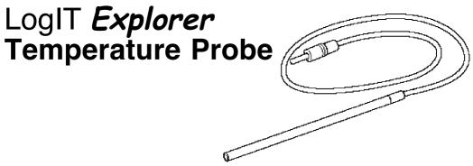
The Explorer Temperature probe has a *maximum* range of -10 to +110°Celsius and is supplied with fitted cable and jack plug. The most sensitive and fast reacting part of the sensor is at the tip of the stainless steel probe.
